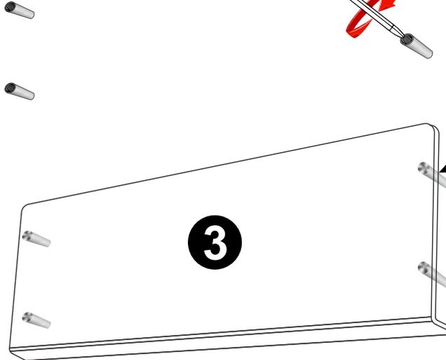
**3** Twist the Standoff Head into position.
