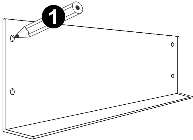
**1** Reverse and place the acrylic rack onto the wall, marking the hole positions.
