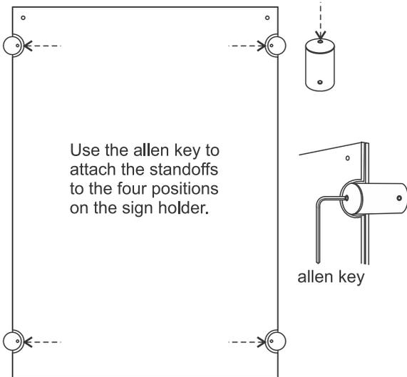
Use the allen key to attach the standoffs to the four positions on the sign holder.
