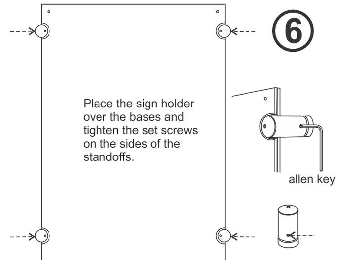
Place the sign holder over the bases and tighten the set screws on the sides of the standoffs.
