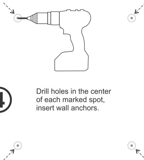
Drill holes in the center of each marked spot, insert wall anchors.
