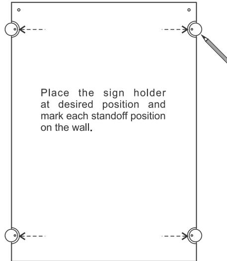
Place the sign holder at desired position and mark each standoff position on the wall.
