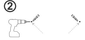
Drill holes in the center of each mark, insert wall plugs.
